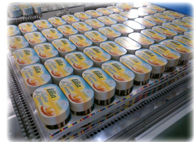
The patented pin system configures to the job layout
