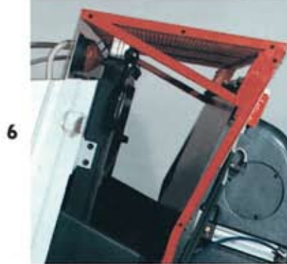
WIDE OPENING VERSIONS. NECESSARY TO INSTALL A DIE-HEATER (FOR HOT DIE CUTTING, FOIL STAMPING AND EMBOSING), OR IF CUTTING RULES HIGHER THAN USUAL ARE EMPLOYED.
